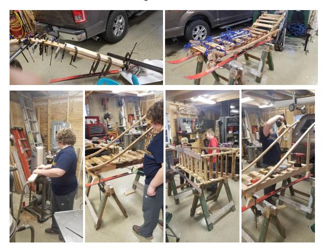
We started the sled by laminating the top rails to give them a bend. Then we cut and drilled all the components for the sled.
